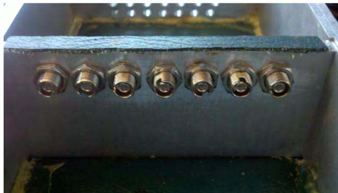
**Figure 4.16** A graphic of the aluminum box where each fiber optic sensor connected and then was fed out of the protected compartment to the data acquisition system.
