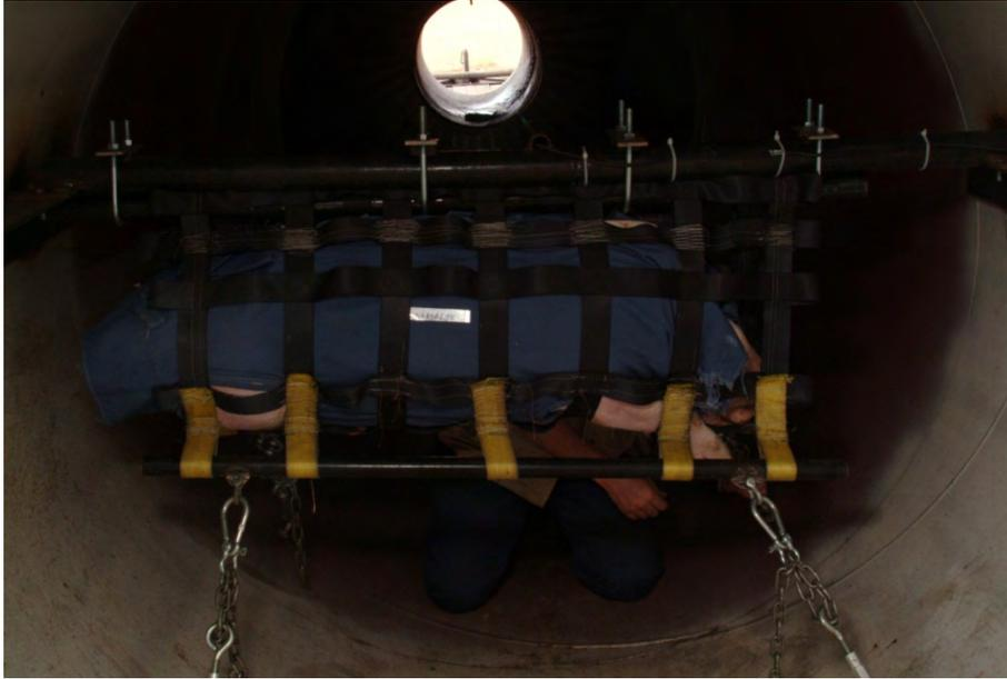
**Figure 4.17** The pig was supported in a canvas sling within the test section. The graphic is facing the explosive end of the tube and the pencil probe can be observed above the support shaft.
